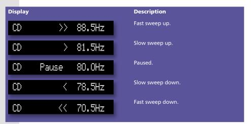
The sine sweep will stop when it reaches 0.5Hz or 200Hz.
